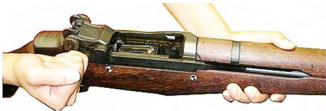
Figure 1. Pulling operating rod
